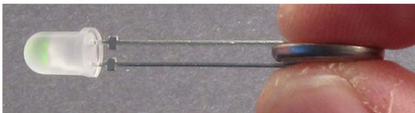
3. Reverse the LED legs so the short leg is on the positive side (+) of the coin battery. Describe how the LED responds and write your observation in your Launch Log.
