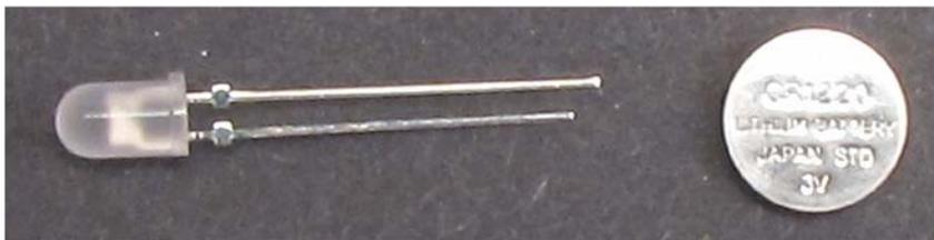
2. Place the long leg of the LED on the positive side of the coin battery with a plus sign (+) stamped on it. The shorter leg will be on the opposite side of the coin battery. Pinch the legs together with your thumb and forefinger. Describe how the LED responds and write your observation in your Launch Log.
