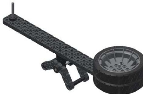
14. Use one hand to move the lever so the tires move up and down.
